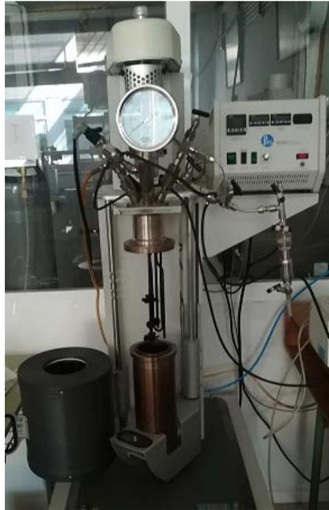
Figura 3.17. Reactor autoclave
