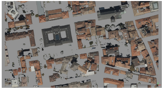
Figure 7. Point cloud after vegetation filtering-S4. Big clusters of vegetation were removed as well as some minor roof points.
