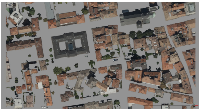
Figure 6. Point cloud after clustering filtering –S3. It should be remarked that still some roofs (corresponding to tents in terraces) and dense vegetation persist.
