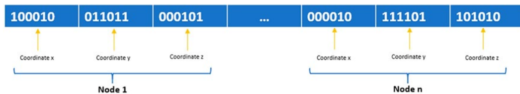
Figure 4.4. Binary coding in GA. Example of association between Cartesian node coordinates and their value in binary coding.
