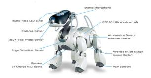
Fig. 1. aiBo robot with its main sensors detailed
