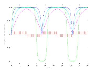
Figure 7: Probability evolution with symmetric sensor models p(occ/obs(t)) = 0.55, 0.6, 0.7 and 0.8.
