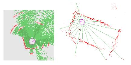
Figure 1: Occupancy grid example (left). Instantaneous sonar readings (right)
