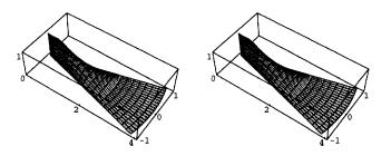
Figure 8: Example of fuzzy sonar models for occupancy (left) and emptiness information (right).
