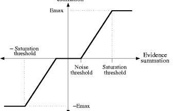
Figure 4: Occupancy state estimation given the accumulated evidence
