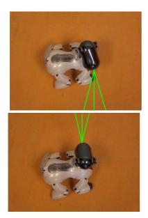
Fig. 5. The robot takes infrared measures when it is faced to corridor with -90, -80, -70, 70, 80 and 90 degrees
