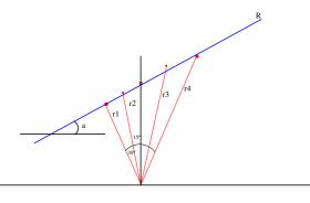
Fig. 6. When we have calculated the 2D points corresponding to sensor measures, we calculate by Minimum quadratic method the line corresponding to an obstacle. The angle a will be used to correct the robot position
