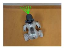
Fig. 4. The robot takes infrared measures when it is faced to wall with -30, -15, 0, 15 and 30 degrees
