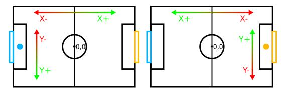
Figure 4. Coordinates given by BICA are team-independent. Position (0,0) marks always the center of the field. Increasing X-axis values get nearer the opponent's goal. Increasing Y-axis values are nearer to the right touchline.
