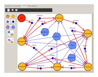
Figure 3. BICA design diagram for a simple goalkeeper behavior. Big yellow circles are *states*, dark blue arrowed spheres are *transitions*. Big, discontinued, purplish blue spheres represent BICA component dependencies.
