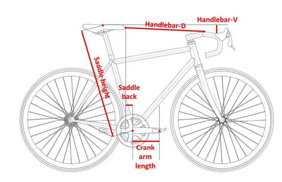
The main bike measurements: saddle height, saddle back, crank arm length, vertical distance between the top of the saddle and the handlebar's brake (Handlebar-V) and distance between the front of the saddle and the middle of the handlebars (Handlebar-D). 211x135mm (150 x 150 DPI)
