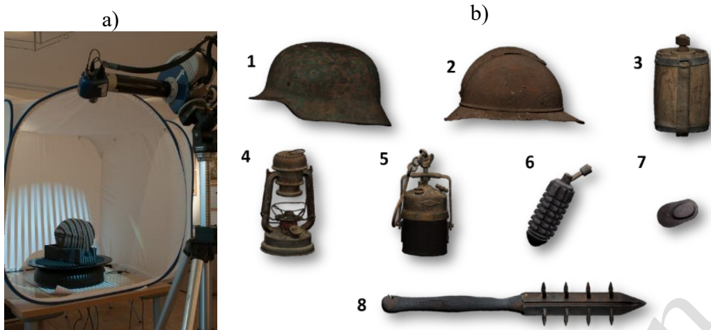
Fig. 8. (a) Scanning an Italian WWI helmet with 3D fringe project scanner. (b) Produced 3D models of war findings: 1) Austro-Hungarian helmet, 2) Italian helmet, 3) Water bottle, 4) Ditmar lamp, 5) Osmeka DB lamp, 6) Hand grenade, 7) Reinforced glasses, 8) Spiked club. All models are freely accessible on the web in the Europeana ( http://www.europeana.eu/portal/en ) and FBK-3DOM ( http://3dom.fbk.eu/repository/portal/portal.html ) portals.
