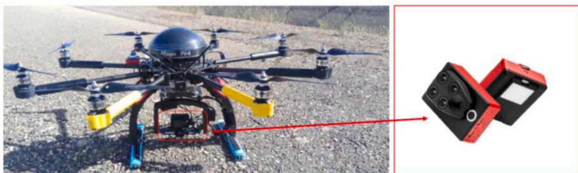
Fig. 4. ATyges FV8 octocopter used in this study to collect UAV multispectral imagery. The red frame indicates the position of the multispectral Parrot Sequoia camera. (For interpretation of the references to colour in this figure legend, the reader is referred to the web version of this article.)
