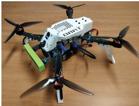
Figure 7. The autonomous UAV prototype implementing the multilevel architecture is presented in this paper. The frame is fully carbon fiber and was designed to host the Nvidia Jetson Nano board and all the additional electronics. Given the increase in weight due to the new elements, the frame was designed to allow the installation of 7-inch propellers.
