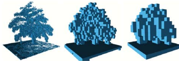
Figure 3. Environment voxelised representation at multiple resolutions [9].
