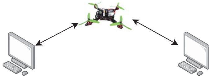
Figure 3. UAV as a mobile relay.
