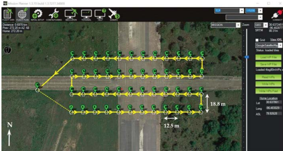
Figure 1. Overview of flight lines and waypoints of the simulated crash scene within Mission Planner.
