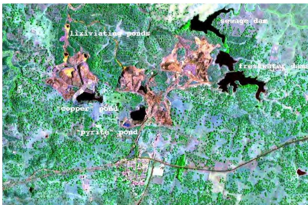
Figure 4.1. False Colour Composite with Hymap channels 11 (0.6029 \mu\text{m} ), 35 (0.9394 \mu\text{m} ) and 109 (2.2103 \mu\text{m} ) of the Las Herrerías mine site (Pyrite Belt, Huelva, Spain), and identification of water bodies according to the traditional mine operation.
