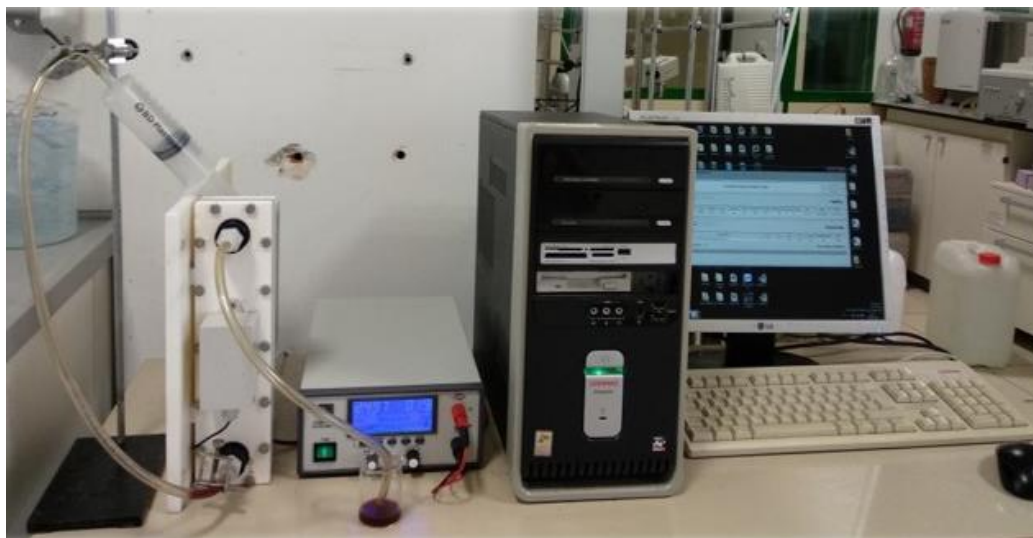
Figure 7.2 Proaqua cell coupled to a power source and controlled by software for wine lees treatment
