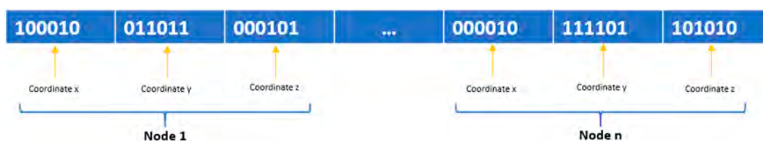
Figure 4. Binary coding in GA. Example of association between Cartesian node coordinates and their value in binary coding.
