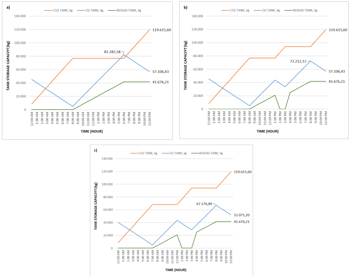
446 Fig. 8 a, b, c. Tank storage capacity operating with a daily discharge cycle: a) continuous operation of 10 447 hours of MES cell; b) discontinuous operation in two 5-hour periods of MES cell with two hours of lag 448 between each period; c) discontinuous operation in two 5-hour periods of MES cell with three hours of lag 449 between each period. The peak capacity value of the oxygen tank decreases as the offline period of the MES 450 cell increases between operating periods.
