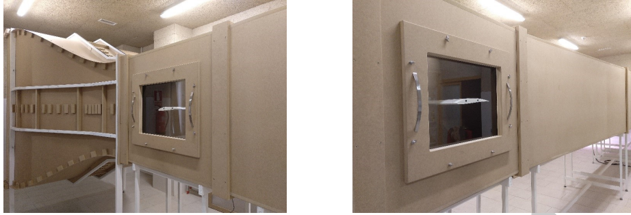
Figure 3: Wind tunnel in which the airfoils were tested. Reynolds values between 4 \cdot 10^4 and 1.1 \cdot 10^5 can be obtained
