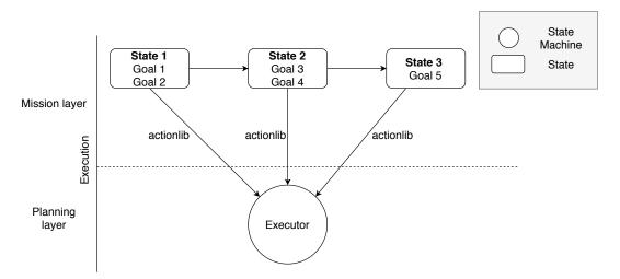
**Figure 3.** Communication diagram of Mission layer, designed as a Finite-State Machine and the Executor from the Planning layer.
