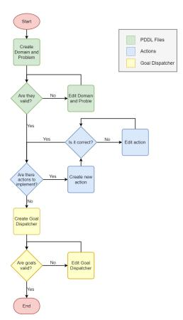
Figure 6. Programming flowchart to create new behaviors using MERLIN.
