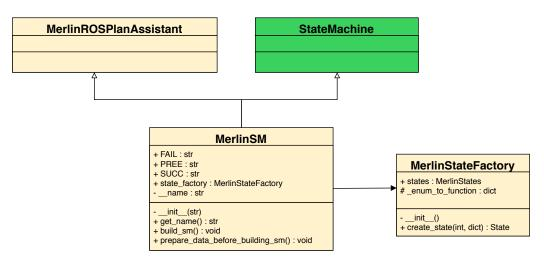
Figure 2. Class Diagram of MERLIN Finite-State Machine.
