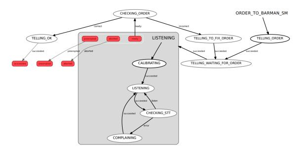
Figure 7. SMACH Viewer presentation of the FSM of the order to barman action.
