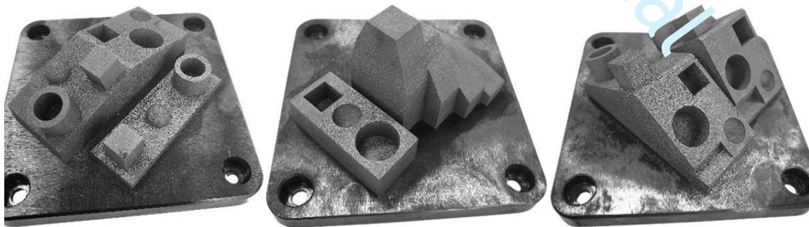
58 Figure 5 Artefacts after the SLM manufacturing process. 59 60
