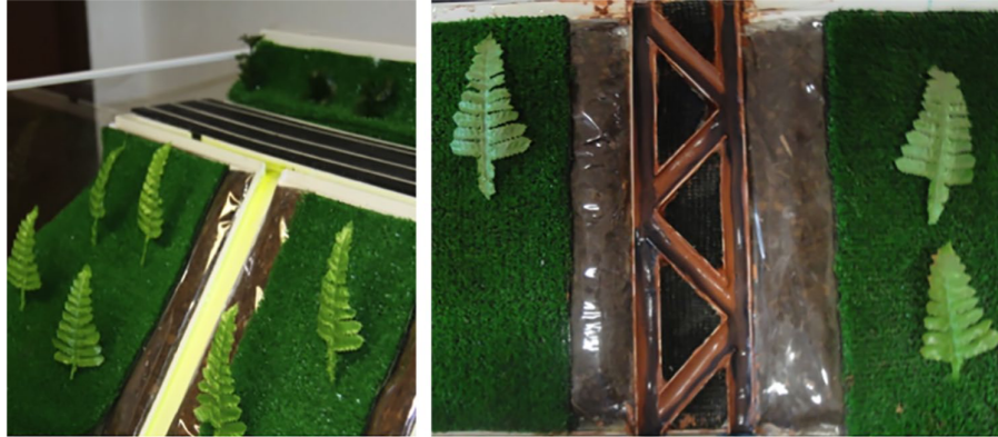
Figure 2. Photographs of the tests performed for the calculation of the average water velocity over the traditional system on polyvinyl chloride (left) and the branched drainage on clay (right).
