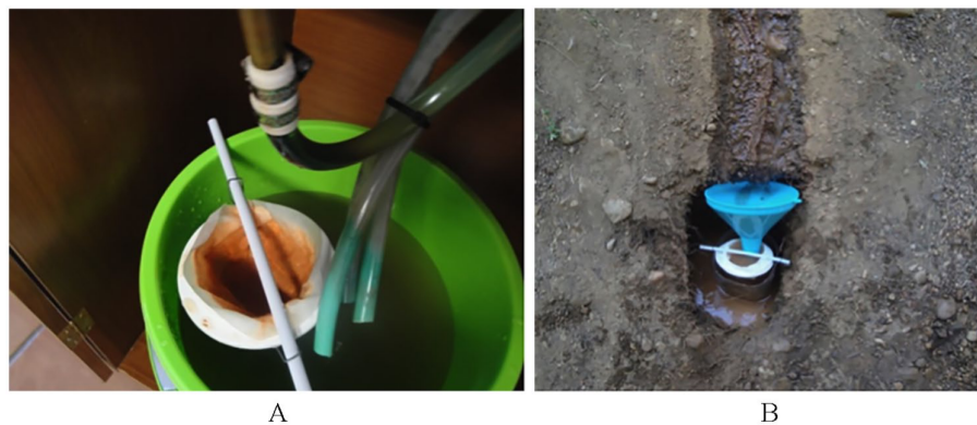
Figure 4. Collection of filters for the soil loss tests in both drainage systems: (A) model and (B) natural terrain.
