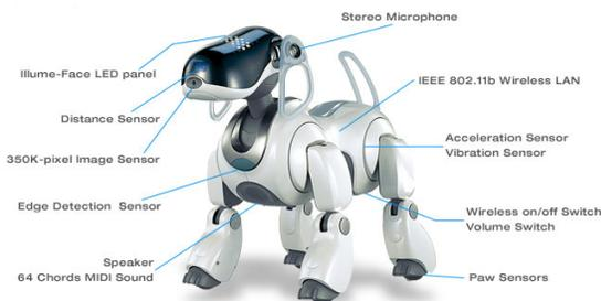
Fig. 1. aiBo robot with its main sensors detailed
