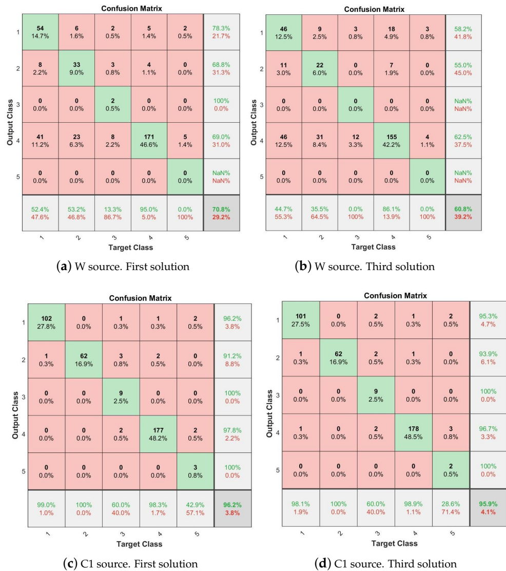
Figure 13. Confusion matrices obtained in the testing phase, for the first (left) and third (right) solution of the Pareto Front, using W and C1 sources.
