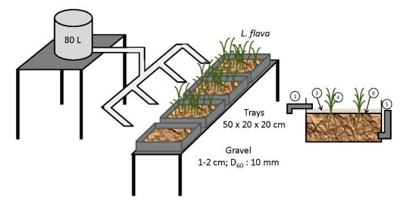
**Figure 8.** Schematic view of experimental setup in the pilot-scale constructed wetland system. Lateral section of planted systems *Limnocharis flava*: 1. Supply pipe; 2. Distribution area (coarse gravel); 3. Gravel 1-2 cm; D60: 10 mm; 4. *Limnocharis flava*; 5. Adjustable output pipe to control water level; 6. Water level. Adapted from [68].
