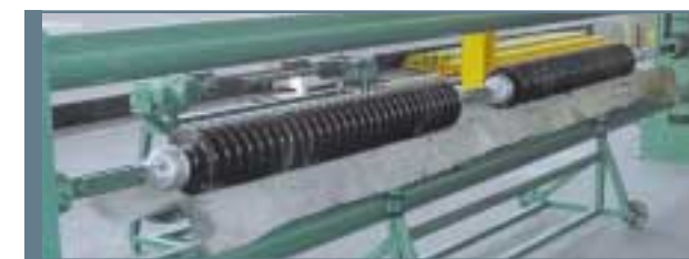
Inspection and Testing of Porcelain Long Rod Insulators according to Standard IEC 60383
