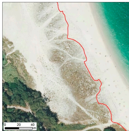
Figure 3. Example of manual shoreline definition on a 2017 orthophotograph.
