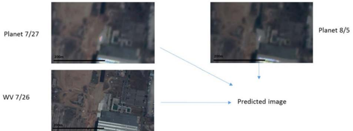
Figure 5. Two Planets images at 27 July and 5 August and one WV image at 26 July are fused to generate a prediction. The prediction is then compared to a WV image collected on 3 August 2017.
