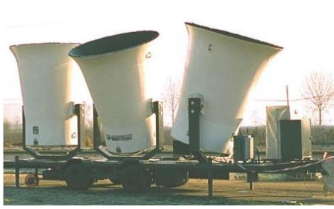
FIGURE 12: ANTENNA SODAR FOR WIND AND TURBULENCE PROFILE MEASUREMENTS UP TO ABOUT 1000 M ABOVE GROUND
