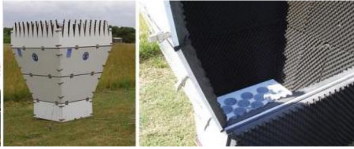
FIGURE 13: PHASED-ARRAY SODAR FOR WIND AND TURBULENCE PROFILE MEASUREMENTS UP TO SEVERAL HUNDREDS OF METERS ABOVE GROUND
