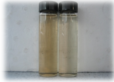
Figure 5.10. Feed solution and permeate samples after membrane operation
