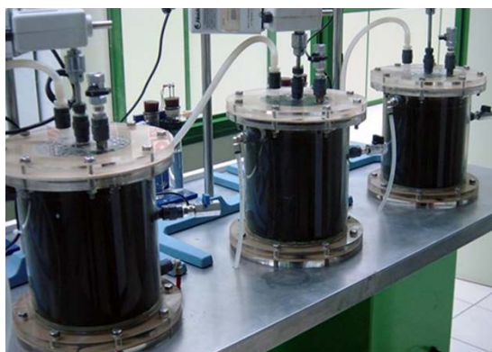
Figure 3.3. The 3-L methacrylate reactors used for the different experiments throughout the thesis.
