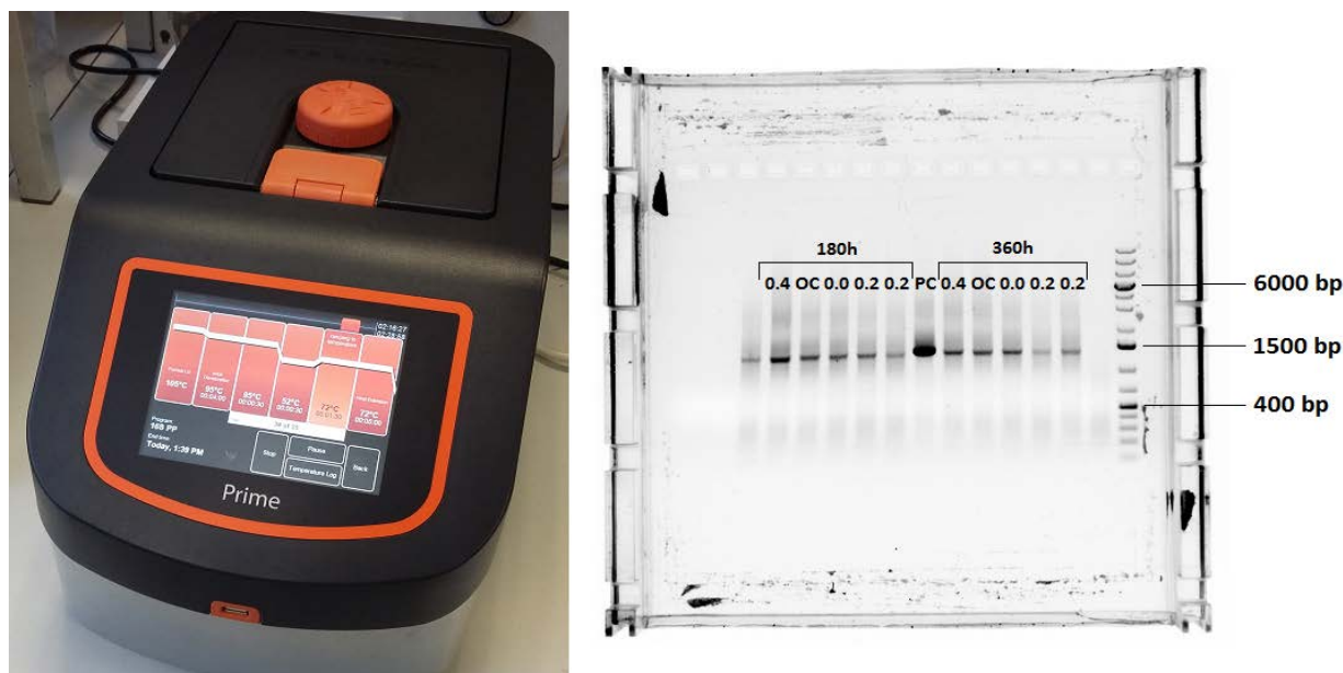
Figure 8.2. Thermocycler used for the PCR, and PCR products in the agarose gel both for 180 and 360 h (PC: positive control).
