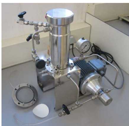
Figure 3.4. Membrane unit and PVDF membrane used for filtration in Chapter 5.
