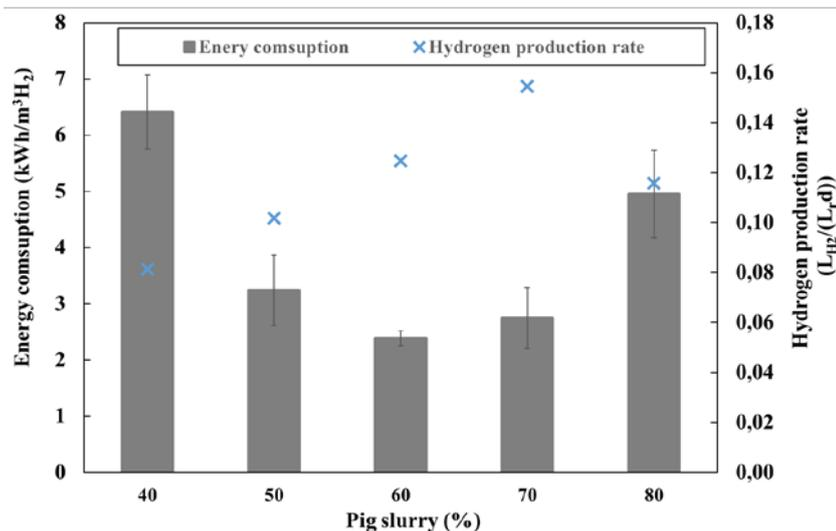
**Figure 2.** Energy consumption and hydrogen production rate as a function of the amount of pig slurry in the feed.
