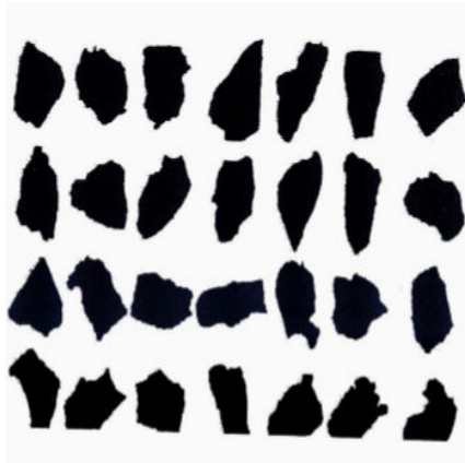
Ilustración 15: Cryogenic rubber particles: Regular pattern shape "cuboid type" (RECIPNEU)
