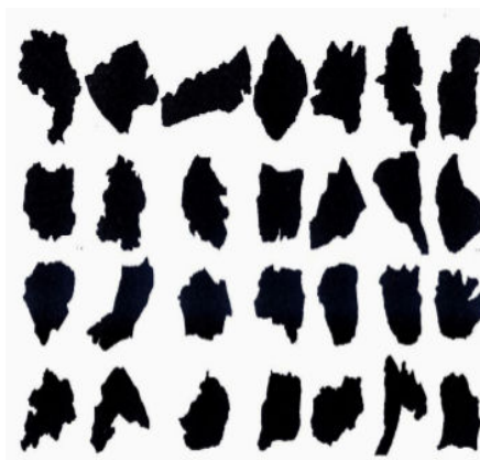
Ilustración 17: Mechanical rubber particles: Irregular pattern shape "spongeous type" (DIRECT-MAT)
