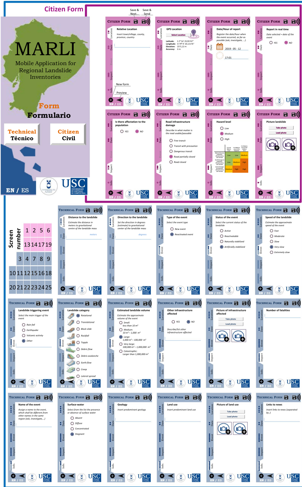
Fig. 1 Interface of MARLI: citizen form (purple box) and technical form (blue box)
