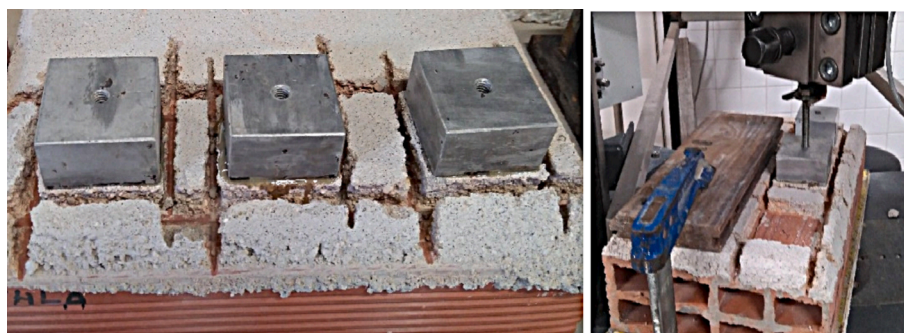
Fig. 2. Square pull-head plates glued on the rendering mortar surface and adhesive test set-up.
