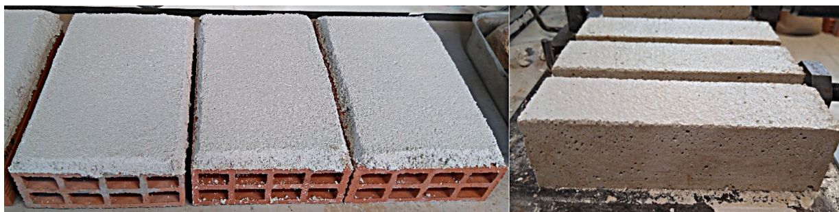
Fig. 1. Examples of the produced mortars as render on brick and prismatic samples.
