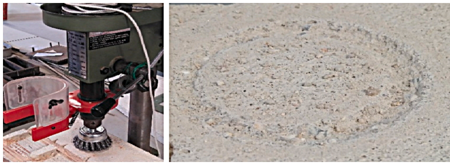
Fig. 3. Abrasion test equipment and relief (left) on a mortar sample.
