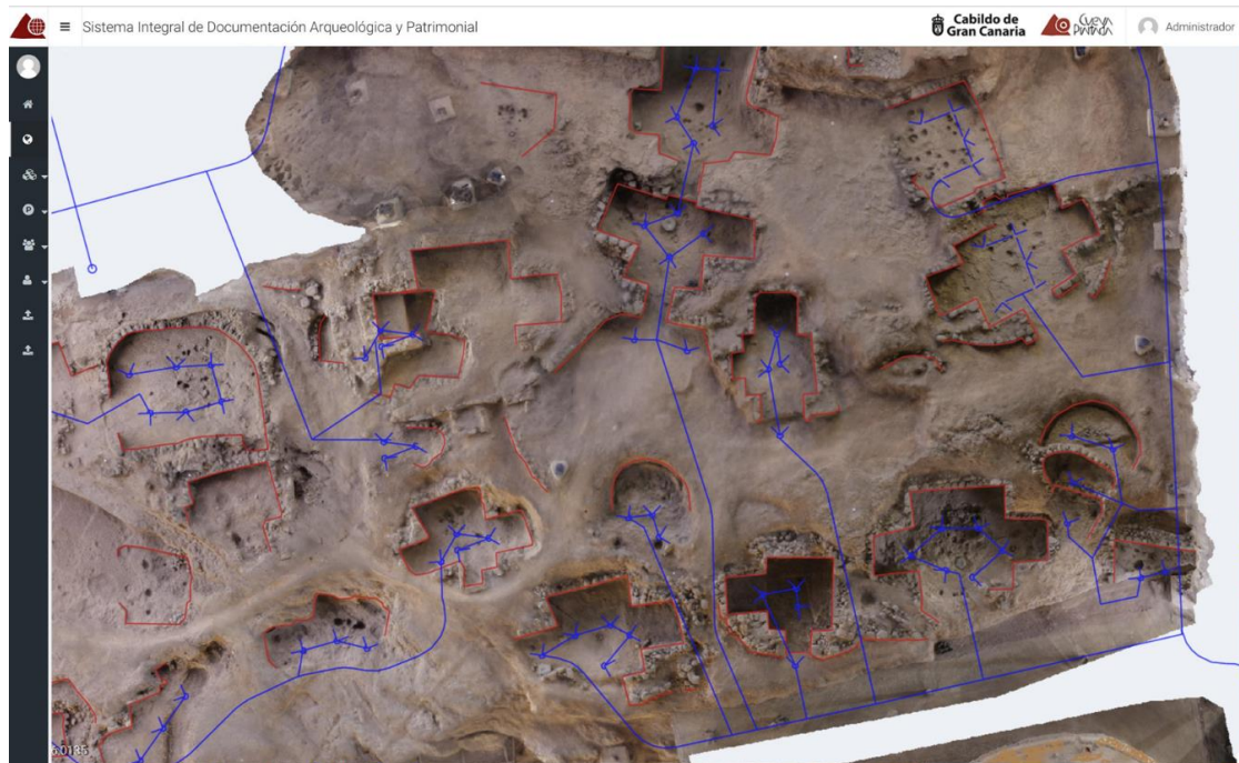
Figure 12. 3D SDI in which the orthophoto of the “Cueva Pintada” (base layer), the delimitation of the different structures (in red) and the lighting infrastructure (in blue) are displayed.
