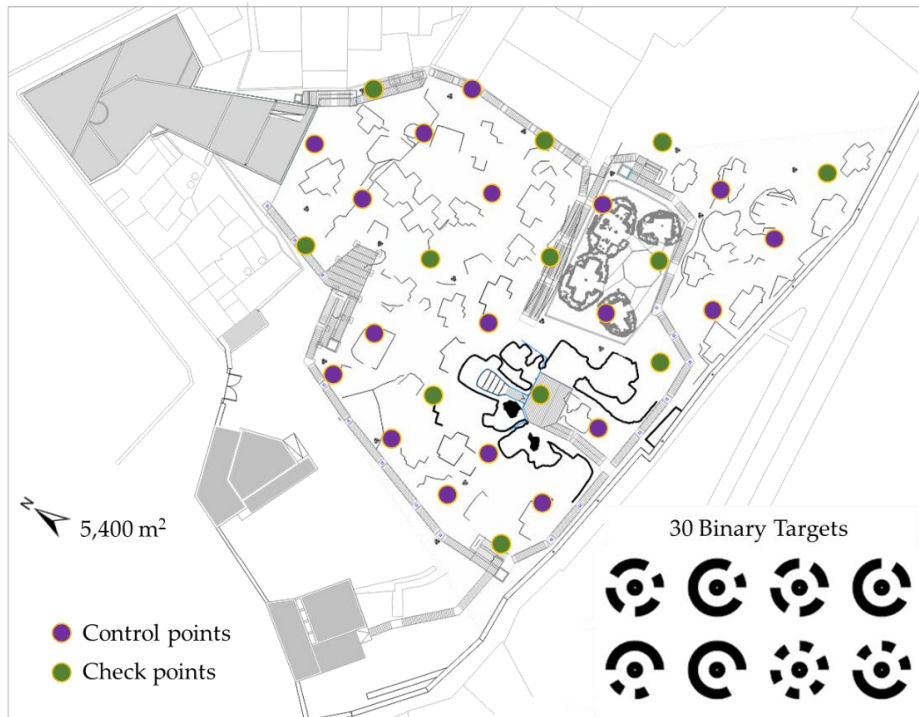
Figure 4. Photogrammetric network designed based on the 12-bit binary targets of 10 cm diameter.
