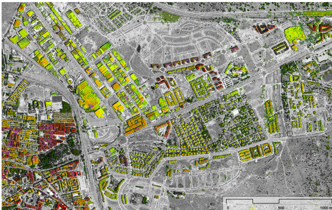
Figure 11. Single-family houses of 1 or 2 floors and the industrial area resulting from the automatic comparison between both flights.
