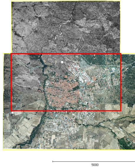
Figure 6. Both point clouds georeferenced in the same reference system, ETRS89, and in the same national cartographic projection, UTM30N. The area under study is marked by the red square.
