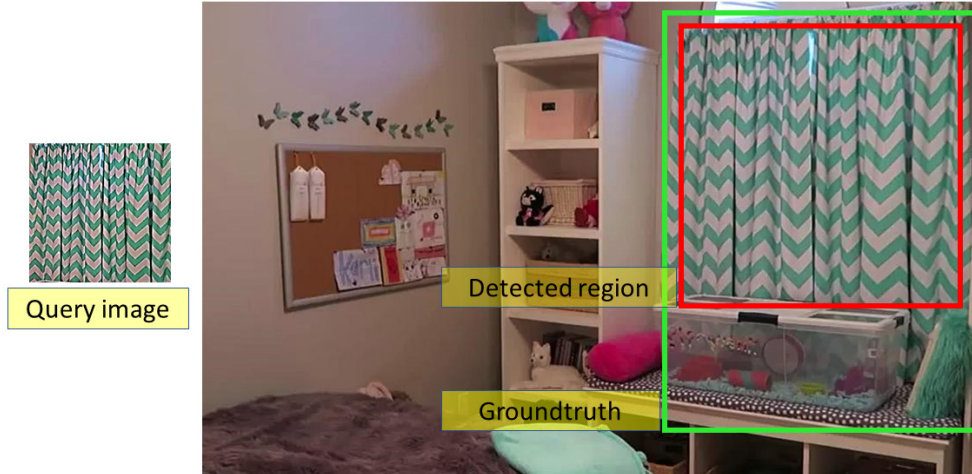
Figure 4.9: The green square shows the groundtruth, and the red one presents the detected region in relation to the query image. Since there is an overlap between both regions, R(i) would be set to 1.
