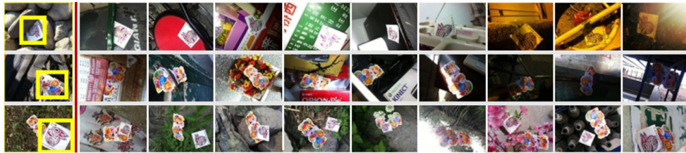
Figure 1.7: Three examples of the result of a CBIR system for instance-level image retrieval. The yellow bounding boxes represent the queried objects, and images in the right are the ground-truth images that contain the query object.
