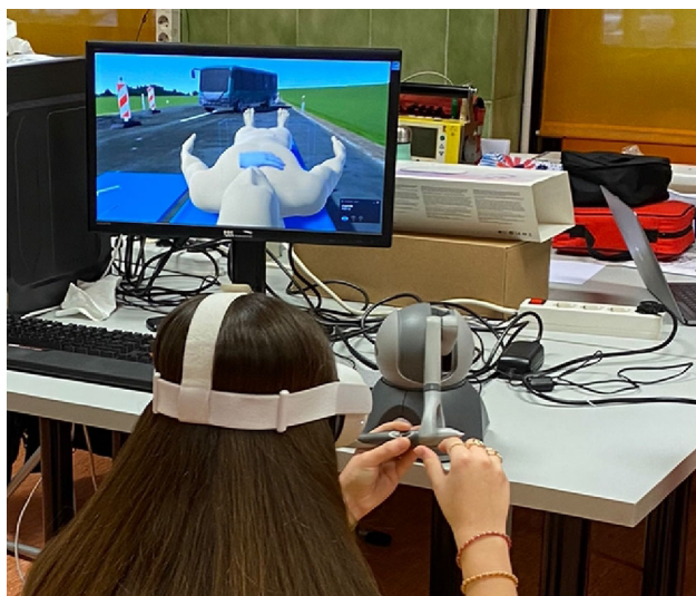
Fig. 1 ParaVR being used. The trainee wears an Oculus Quest 2 HMD connected to a computer and interacts with the simulation using the Touch haptic device
