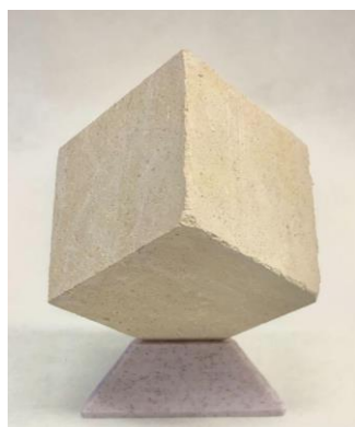
Figure 1. Boñar (Spain) limestone specimen as delivered from quarry (50 mm edge cube).
