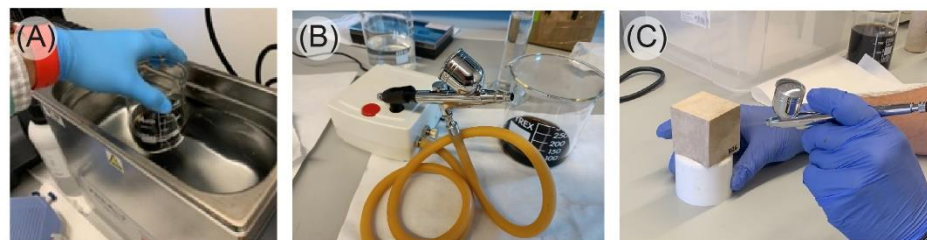
Figure 3. Specimen preparation: (A) ultrasonic-bath-based dispersion of GO, (B) airbrush connected to the pump, and (C) airbrush application.
