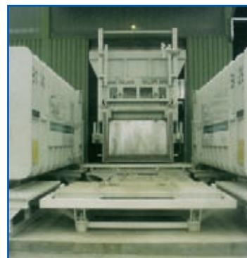
MP 6000 with traversing lifting trolley and weighing system
