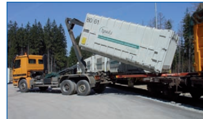
Loading of ACTS containers onto railway waggons
