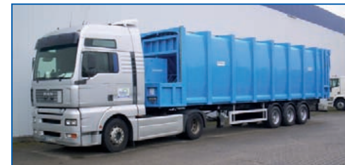
Push-out trailer 60m 3 , payload approx. 20 tons
