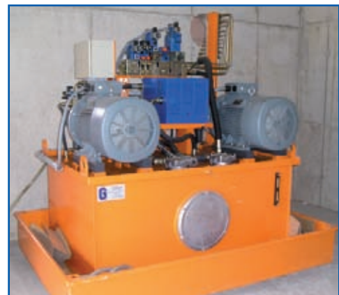
Twin-pump power pack
