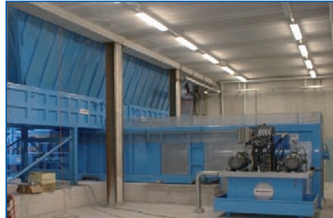
MP 6000 with 2 lateral pushers and 3 parallel dumping places
