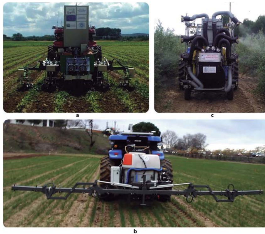
Fig. 4 – Implements working: (a) Flaming and row cultivator, (b) Patch sprayer, and (c) Canopy sprayer.
