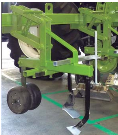
Fig. 13. Tillage tool with the flaming and row crop cultivator implement.
