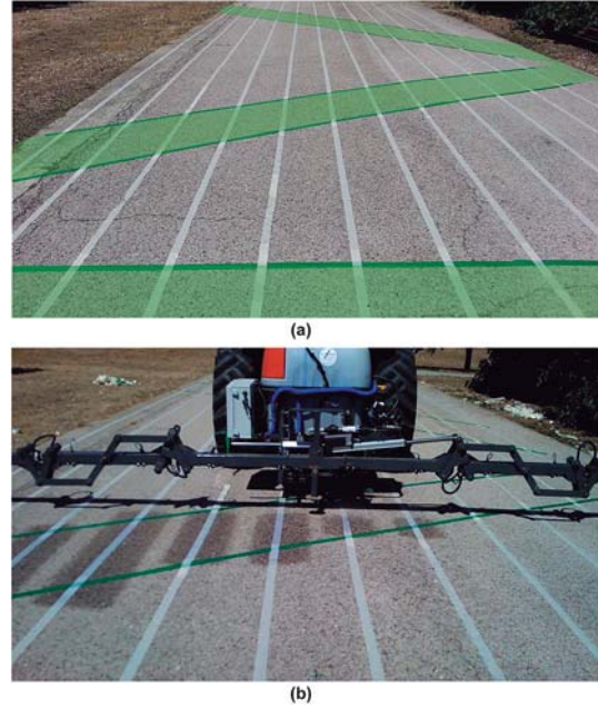
Fig. 7 – Test pavement: (a) general vision, and (b) the system working over the simulated weed patch.
