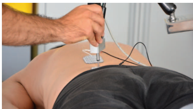
Figure 2. Tensiomyography electrodes and digital displacement transducer placed perpendicular to the muscle belly.
