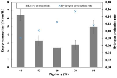
**Figure 2.** Energy consumption and hydrogen production rate as a function of the amount of pig slurry in the fed.
