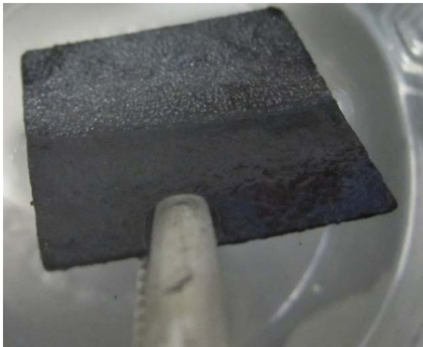
Figure 4.2: Carbon paper electrode with air bubbles after pre-treatment
